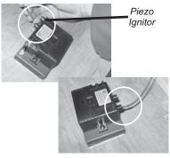
Insert both the ground wire and the DC sparker generator wire through the hole of the DC spark heat shield.
